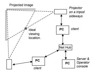
Figure One: Overhead Diagram of the two-screen UT-Cave.
